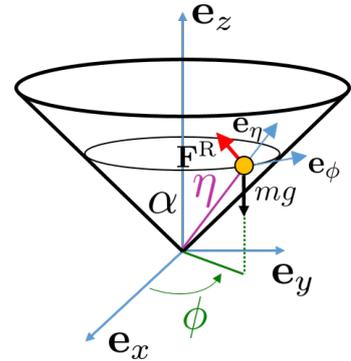
$$\begin{aligned}x(\eta, \phi) &= \eta \sin(\alpha) \cos(\phi) \\y(\eta, \phi) &= \eta \sin(\alpha) \sin(\phi) \\z(\eta, \phi) &= \eta \cos(\alpha).\end{aligned}$$
