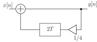
c)  $H(z) = z^2 \left[ \frac{2}{z-1/2} - \frac{2}{z+1/2} \right]$  (Partialbruchzerlegung)
