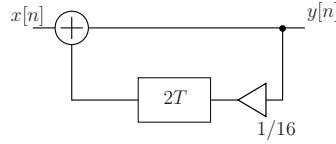
c)  $H(z) = z^2 \left[ \frac{2}{z-1/4} - \frac{2}{z+1/4} \right]$  (Partialbruchzerlegung)
